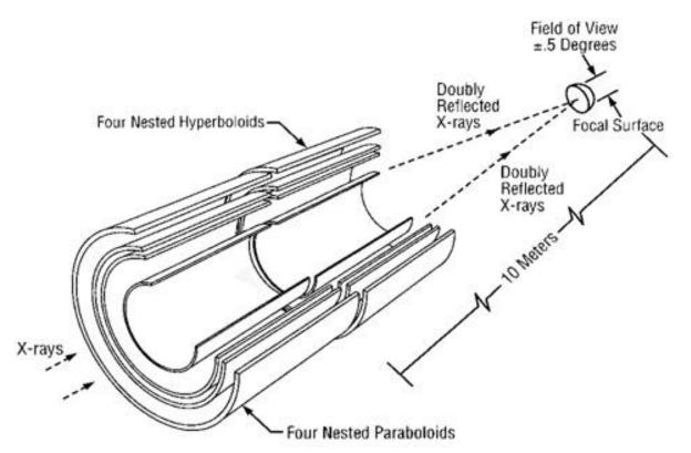
The High-Resolution Mirror Assembly is contained in the cylindrical "telescope" portion of the observatory. The entire length of the telescope is covered with reflective multi-layer insulation that assists heating elements inside the unit in keeping a constant internal temperature. By maintaining a precise temperature, the mirrors within the telescope are not subjected to expansion and contraction – thus ensuring greater accuracy in observations.
